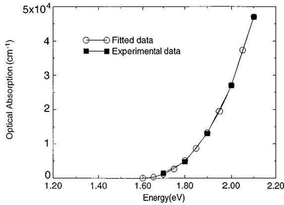
FIG. 3. The optical absorption as a function of energy on a linear-linear plot for the experimental and fitted data on *a*-Si:H.
