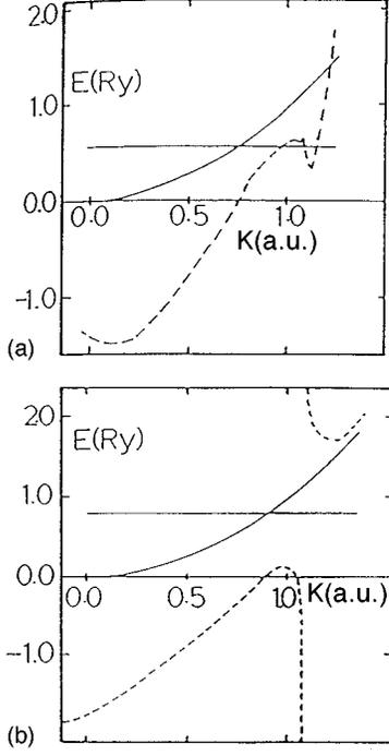
FIG. 1. The behavior of  $k^2 + \Gamma_R(kE)$  as a function of  $k$  (a) for an energy ( $E$ ) just outside the gap, and (b) for an energy within the gap. The horizontal line denotes the energy and the solid curve is the free-electron form ( $k^2$ ).
