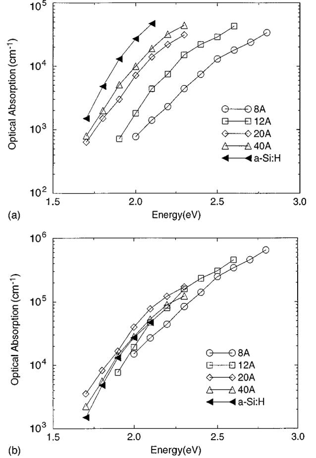
FIG. 2. The optical absorption as a function of energy on a linear-log plot: (a) unscaled data and (b) scaled data for thin layers and bulk *a*-Si:H. The symbols denote points read from the original data for the purpose of rescaling.
